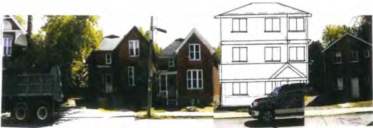
B. Elevation in context, without a garage fronting University Ave but with a hip-slope roof and a canopy. Assuming the building is set-back 5 feet from the street, the latter acts as a kind of porch with parking confined to the rear yard. If the building is set-back 20 feet from the street, there is a canopy extending over half that distance and sheltering 2 cars plus a garage door.
