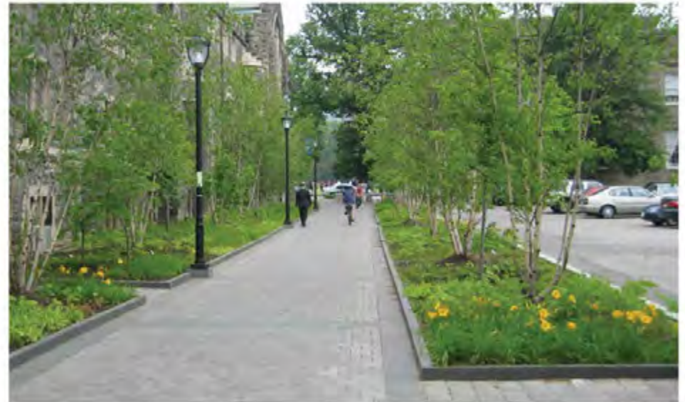
Pedestrian pathway separated from parking by planting (University of Toronto; source: Urban Strategies)
