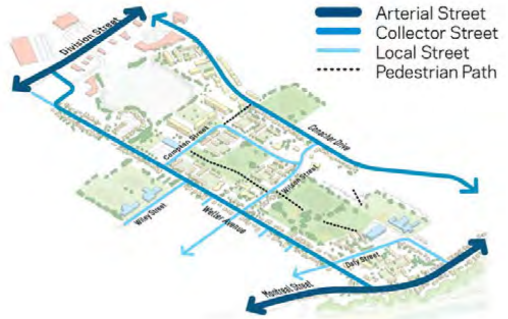
The above diagram illustrates that existing local streets and pedestrian paths do not complete a well connected network.
