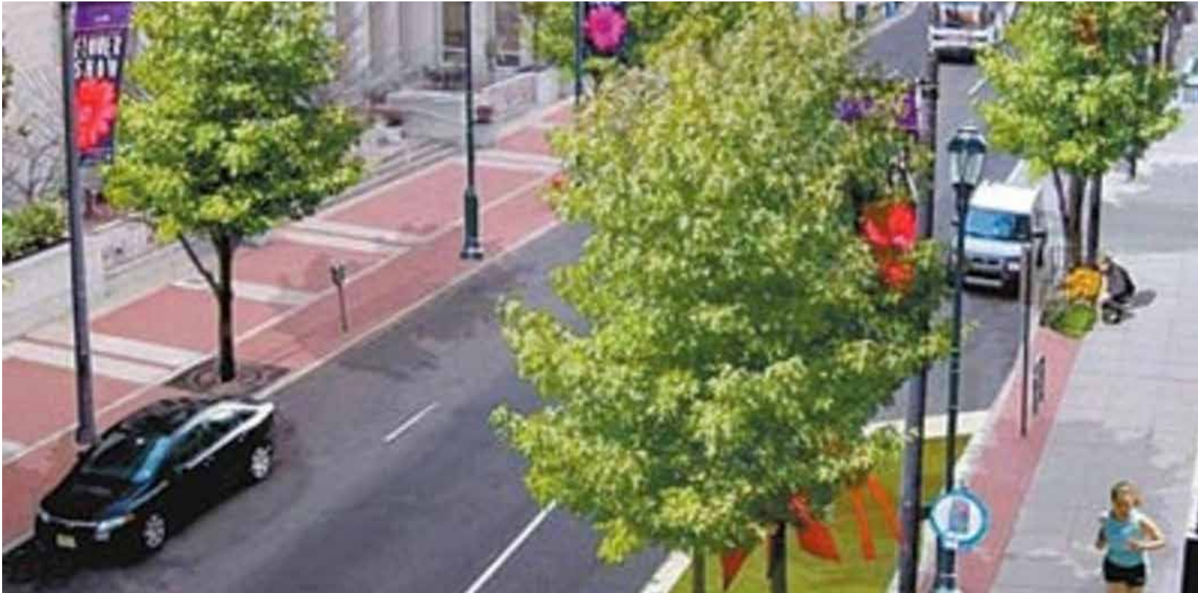
Figure 3-16: Example of layby parking and planting bump-outs to create on street parking spaces
