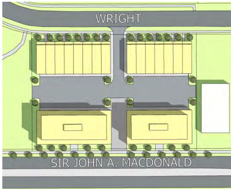
Figure 3-5: Arterial Road Concept: Sir John A Macdonald (right of way) width varies, desired 36.6m as per Official Plan) and Bath Road (desired ROW width 42.0m per Official Plan)
