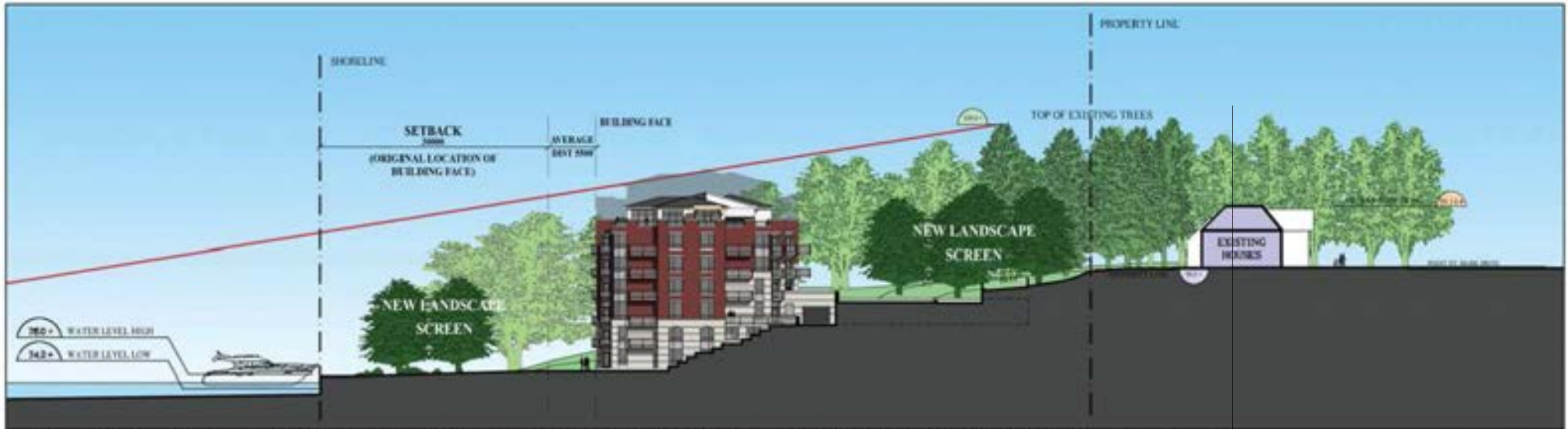
EAST-WEST SECTION SHOWING CONCEPTUAL PROPOSED DEVELOPMENT AND LANDSCAPE SCREENING STRATEGY AT 10 YEAR GROWTH SCALE 1:500
