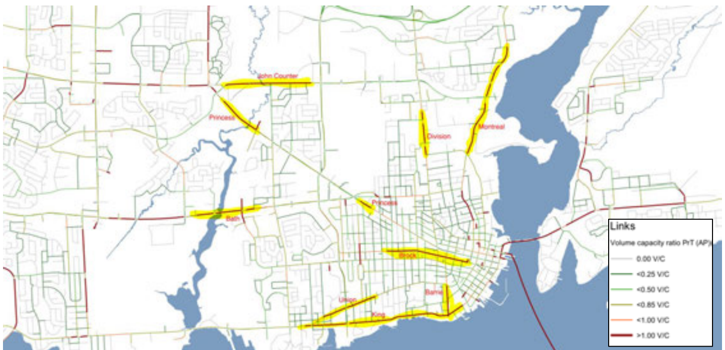
Figure 3: V/C Ratios from 2014 Transportation Forecasting Model (Source: City of Kingston)
