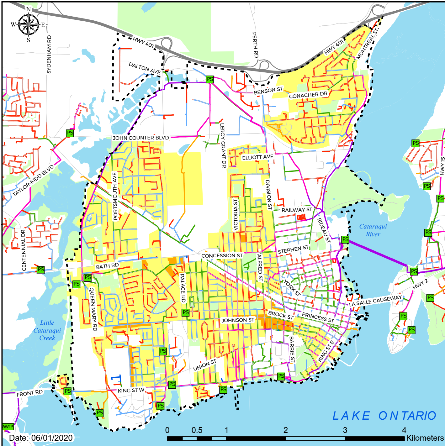
Figure 4 Kingston Existing Sanitary Pipe Diameter
