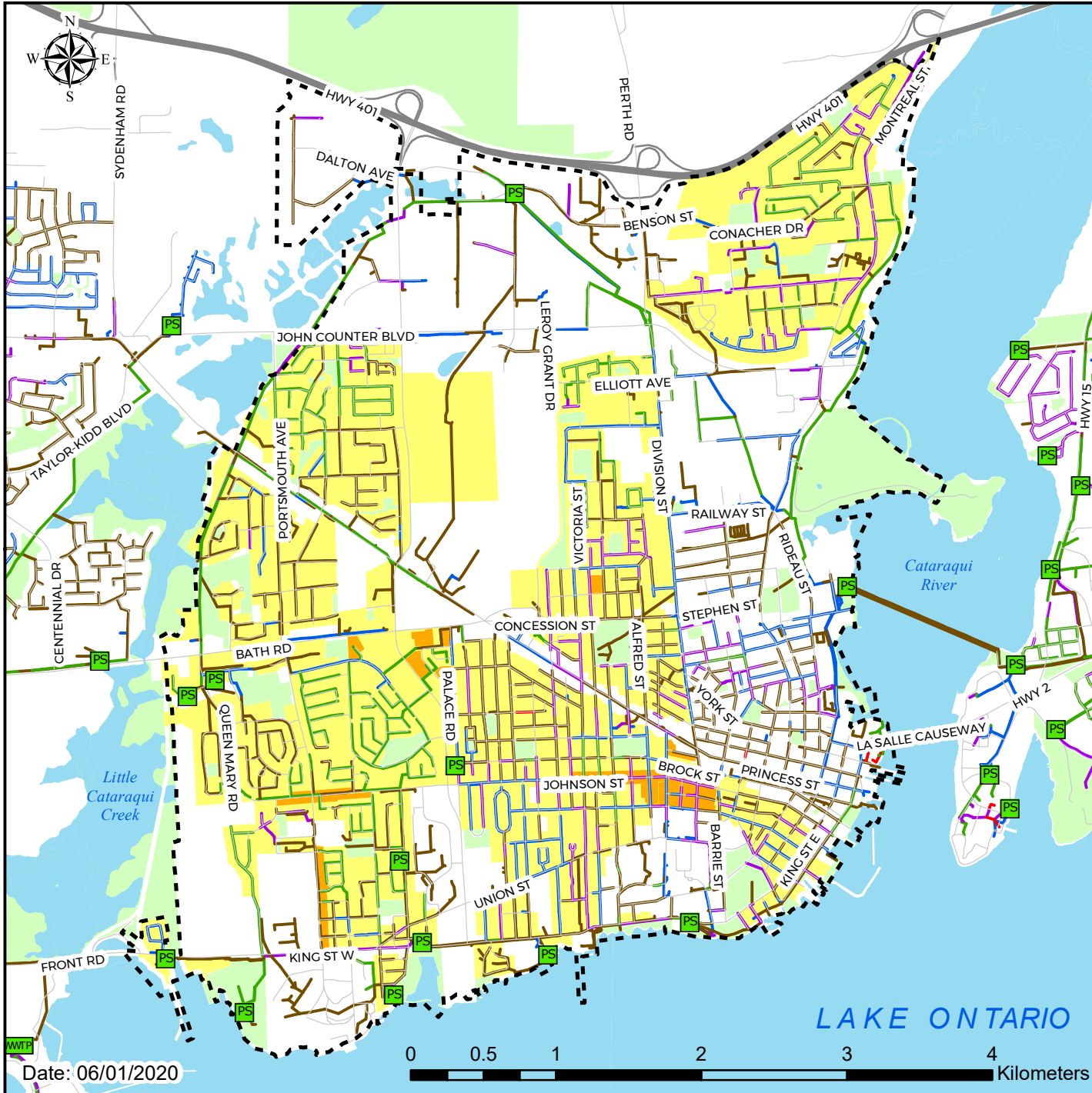
Figure 8 Kingston Existing Sanitary Pipe Installation Year
