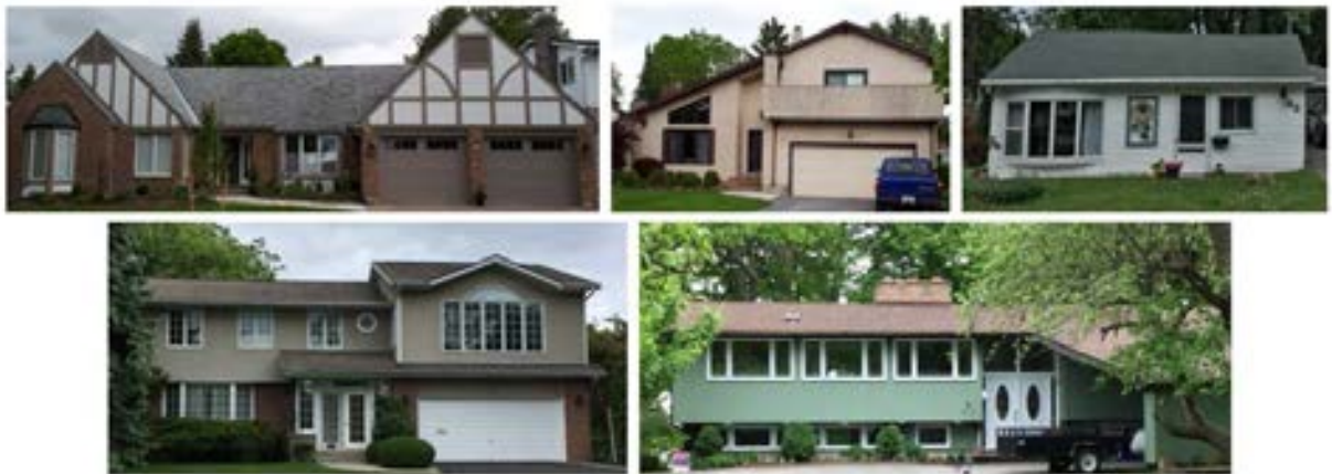
Figure 11: Examples of window placement complementary to the architectural style and front door orientation to the street
