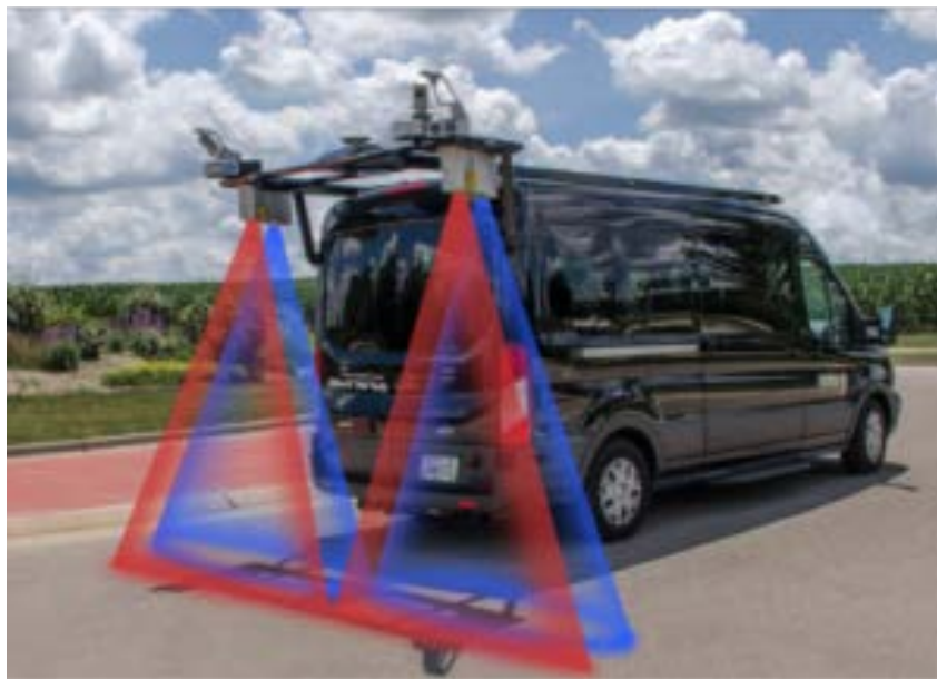
Figure 1.0: Specialized vehicle to collect distress data
