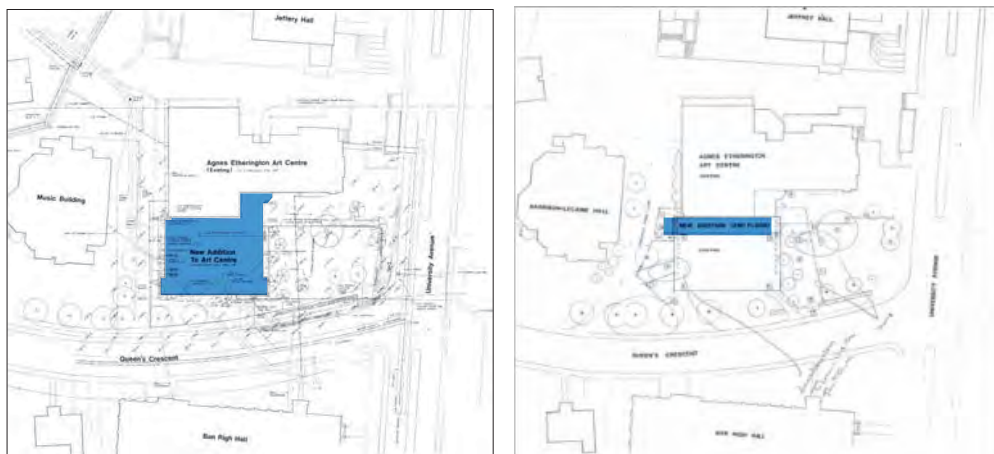
3. 1974 (left) and 1989 (right) Site Plan drawings with additions indicated in blue (Source: Mill, Ross, and Sadhina Architects; and Marshall, Merret, Stahl, Elliott, Mill, Ross Architects, annotated by ERA).
