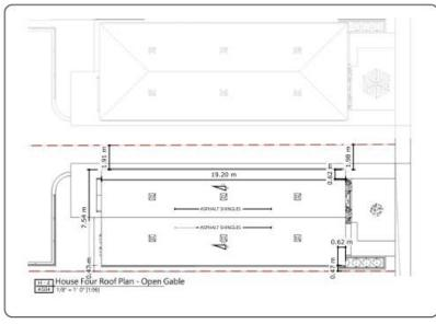
BOOF SCHEMATIC DESIGN PLAN NOTES TO BE CONFIRMED WITH STRUCTURAL AND TRUSS ENGINEER **BUILDING ROOF** ILDING ROOF PITCH 4/12 - HIP ROOF ASPHALT SHINGLES AND CAPPING 2-0" SOFFIT - FINISHED TO MATCH FASCIA BOARD 12" (SIMILAR) FASCIA BOARD - GRANITE GREY EAVES AND DOWNSPOUTS TIE INTO STORM MATCH FASCIA AND SOFFIT COLOUR/FINISH FRONT [EAST & WEST] BROW ROOF (OVER MAIN ENTRYWAYS) [POTENTIAL TO HAVE BROW ROOF ACROSS EAST FACADE WITH COLUMNS (WOOD TONE)]
