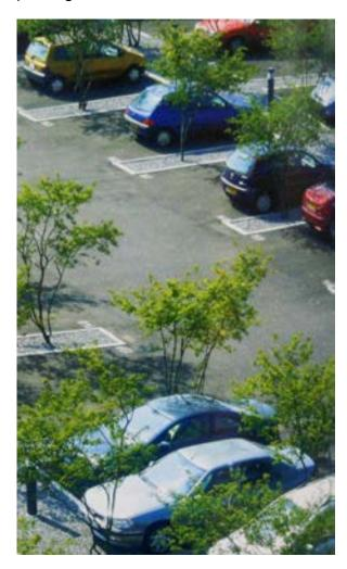
Figure 6-5: Decorative stone is used as a permeable surface treatment. Trees are used to shade vehicles and pedestrians, and to break up the continuity of the surface parking area.
