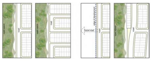
Figure 4-1: New communities should create a positive connection between development and open spaces. Streets adjacent to parks and open spaces can be designed in a number of ways to maximize access and create a vibrant and active streetscape.
