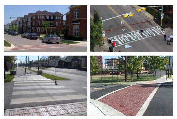
Figure 5-16: Crosswalks are clearly-defined, properly graded and connected to the sidewalk network. Defined crosswalks remind users of pedestrian priority.
