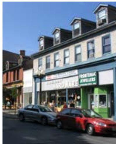
**Figure 6-1:** Parallel on-street parking is preferred over perpendicular or angled parking to minimize the overall width of the street and to optimize sight lines.
