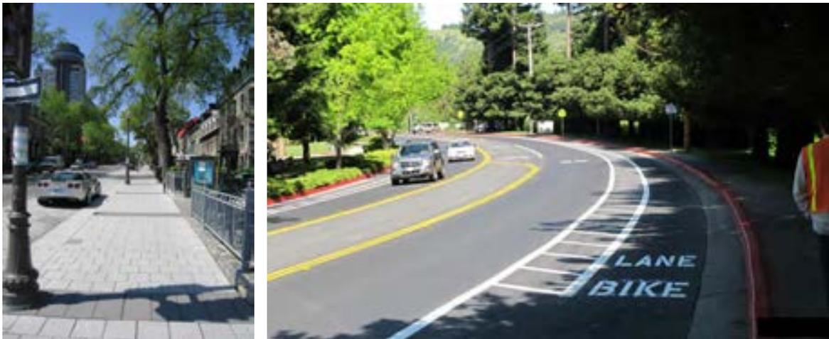
**Figure 5-2:** (Left) On Collector Roads, on-street parking should be provided on both sides of the street where adjacent to commercial or mixed use areas. (Right) Provide appropriate cycling infrastructure on Collector Roads.
