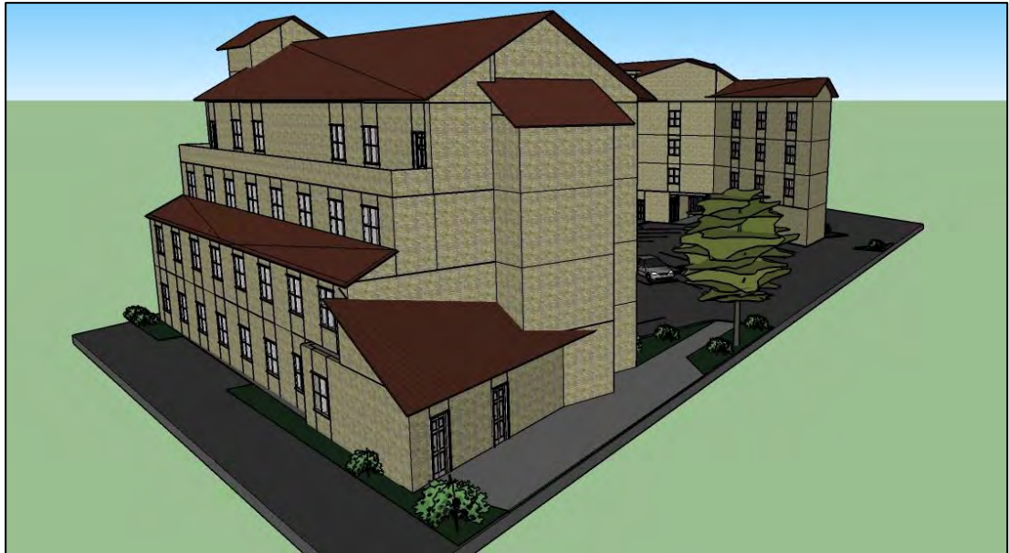
Figure 21: Rendering of south elevation showing stepping back of third and fourth floors (Phase 2).
