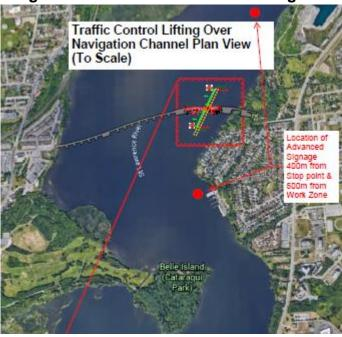
Image of work over navigation channel and the traffic control measures (red is spotter boats)
