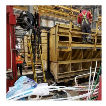
**Step #3 Pouring concrete into the form of the girder:** Once the metal forms are squeezed and in place, concrete gets pumped into the space between the two steel forms with the reinforcing steel in the middle. After pouring, the concrete cures in a temperature and moisture controlled room for about seven days.
